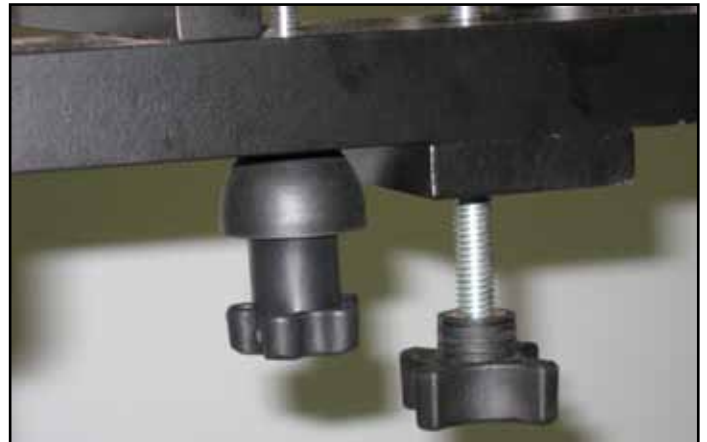
Old style: A short weak pivot arm produces too much wiggle and angular rotation
