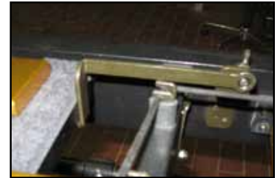
Old style: A short weak pivot arm produces too much wiggle and angular rotation
